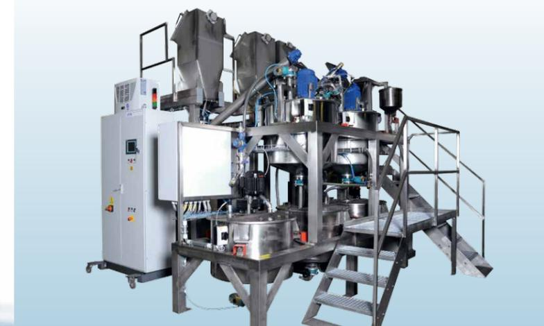
Depending on the application, our systems can be of explosion-proof (gas/dust) or acid-proof design. We consider your individual requirements and build customised agitators for you – for homogenising, emulsifying, aerating, grinding, suspending, dispersing or mixing and dissolving your solid and liquid substances.
